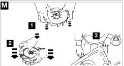
To Refit the Fan and the Cutting Head (M)
